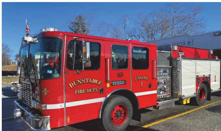
Figure 1 2021 HME Fire Engine 1250 GPM Pump, 1000 gallons of water, 30 gallons of foam
